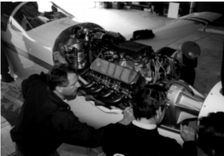
The Legend's big block V-8 and SRU are packaged in a snug and sturdy cowl which removes relatively easily.
