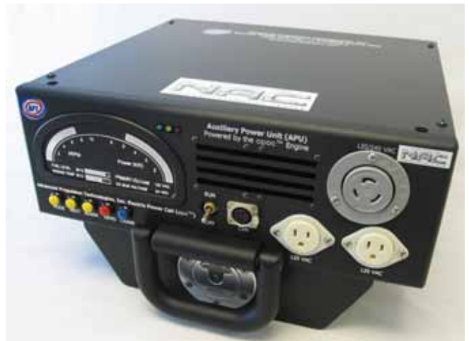
Designed by Advanced Propulsion Technologies, this briefcase-size 5-kW generator has five times the power density of a conventional generator. The portable auxiliary power unit is appropriate for delivering in-vehicle power as well as plug-in exportable power.
