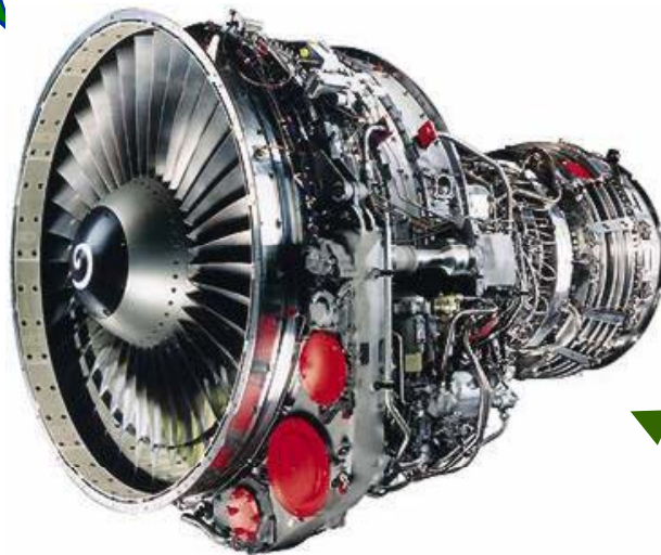
CF6 Aero Engine (core of LM2500 engine)
