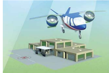
Figure 23. Intra-Urban Ultra Mobility Mission High-Speed VTOL Air-Taxi Concept (5 place, 300 mph cruise, 400 mile range, VTOL)
