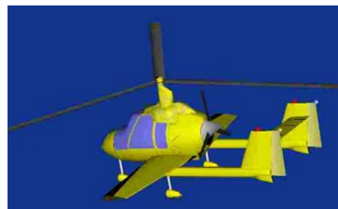
Figure 21. Georgia Tech/NASA Hanson Autogyro Ultra Mobility Mission Low-Speed VTOL Concept
