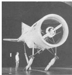
Figure 18. Lippisch Aerodyne Concept in the NASA Ames Wind Tunnel in the 1960's
