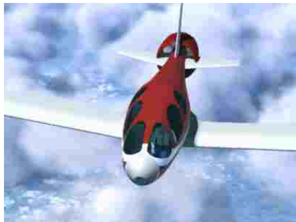
Figure 14. Rural/Regional Next Generation GA High Performance Mission Concept (5 place, pressurized, turbocharged, 300 mph cruise, 500 mile range, near all weather, $125,000 vehicle)
